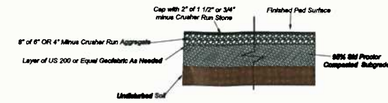
Typical Pad Cross-Section NTS
