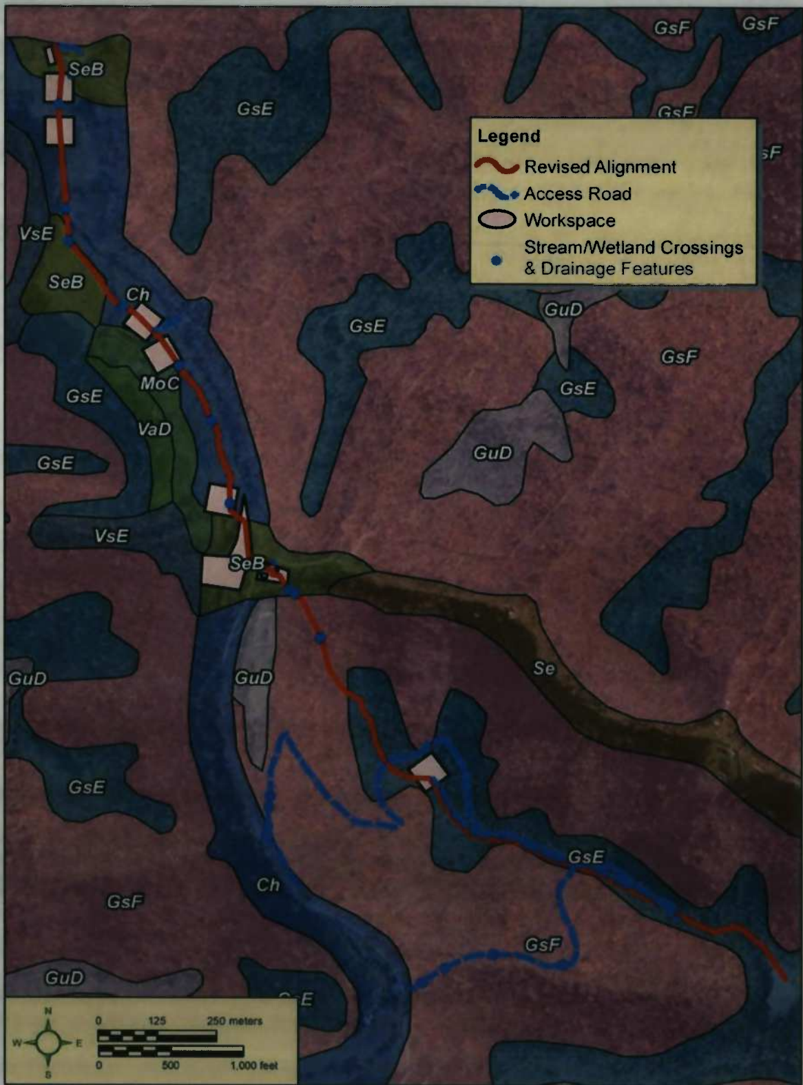
Figure 6. Soils map depicting Project and areas mapped as alluvial and colluvial soils.
