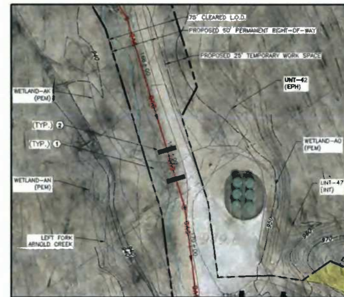
DETAIL X - UNIT 42 (EPH) STREAM CROSSING
