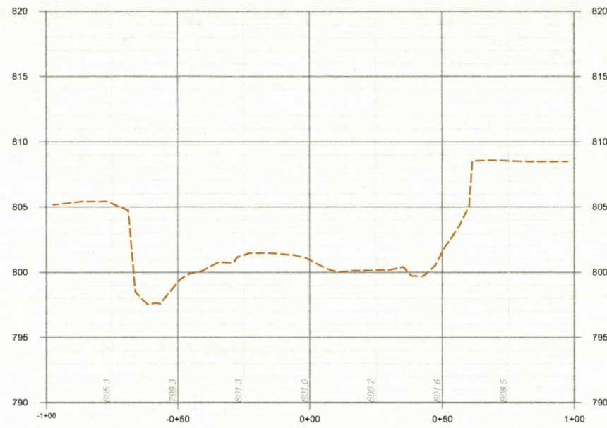
BUCKEYE CREEK CROSS SECTION 2 STA. 1+75.86
